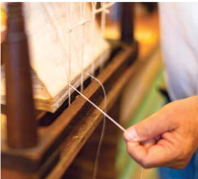
Eberth sews together the gatherings with cords, which are later attached to the boards beneath the cover.
